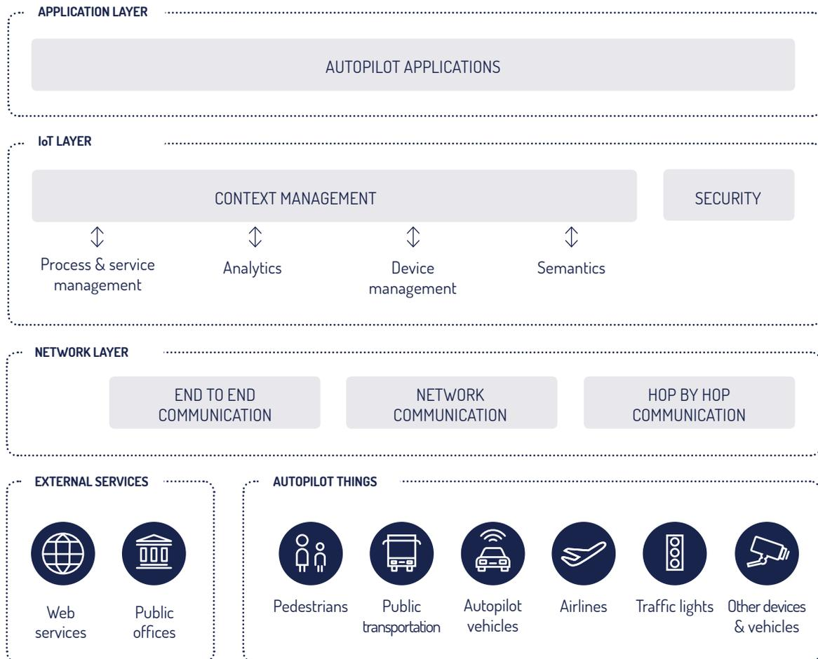
The AUTOPILOT reference architecture is developed to leverage autonomous driving and innovative mobility services based on open IoT platforms. The AUTOPILOT architecture is used as a common framework to realise IoT-based automated driving use cases. IoT components are deployed at several permanent pilot
