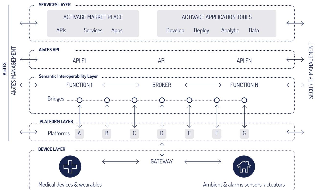
ACTIVAGE architecture is designed to serve as common framework to build interoperable smart living solutions in the form of apps, software tools and services that can be deployed, extended and replicated at deployment sites across Europe. In other words, to allow future support of any
