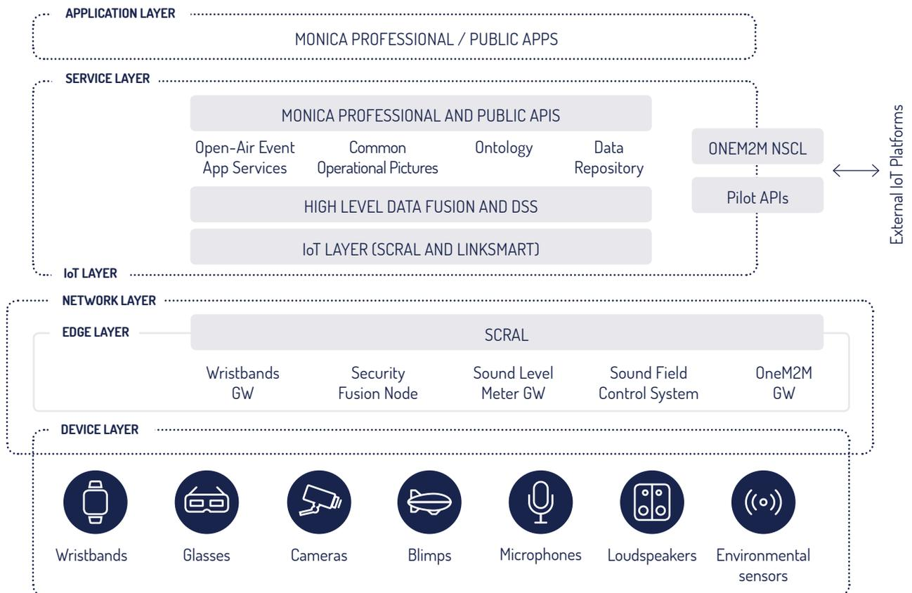
The MONICA IoT platform consists of control systems which monitor the data collected and which can perform automated actions. Components
