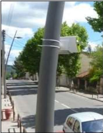
Possibility of bundling the sensor regardless of the shape or diameter of the pole
