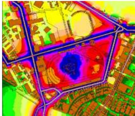
**Figure 5: Propagation example: Forward Model (e.g. Nord2000): Predicts sound field according to input parameters**
