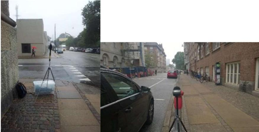
Figure 22: Measurements outside Tivoli using a front-end (left) and a SLM (right)
