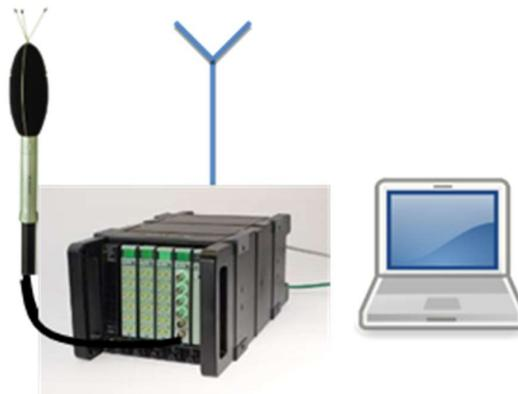
**Figure 21: Setup using front-ends for synchronous data, including a GPS antenna for synchronization.**
