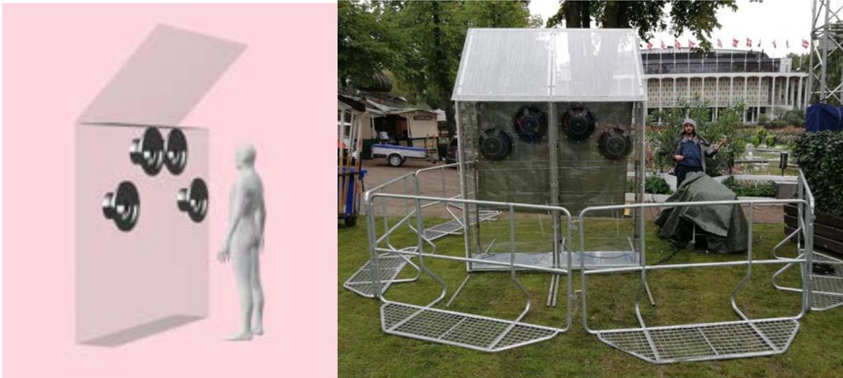
Figure 24: Prototype of the Quiet Zone System tested at the Tivoli pilot site. The controller and the error microphones are not shown here.
