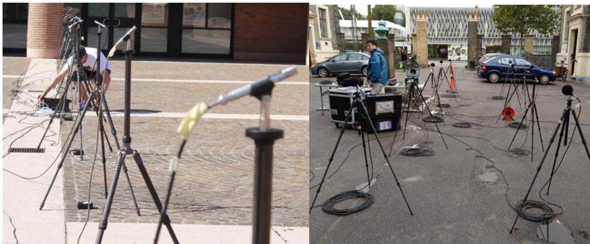
Figure 49: Non-wired measurements of Transfer Functions at KFF2018 (Left) and Tivoli 2018 (Right). An array of 10 microphones where connected to a B&K frontend equipped with GPS time synchronization.
