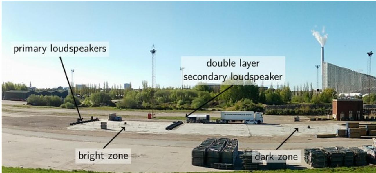
Figure 16: Photo of large scale outdoor experiment setup. The experiment took place at Refshaleøen in Copenhagen, a former industrial area.
