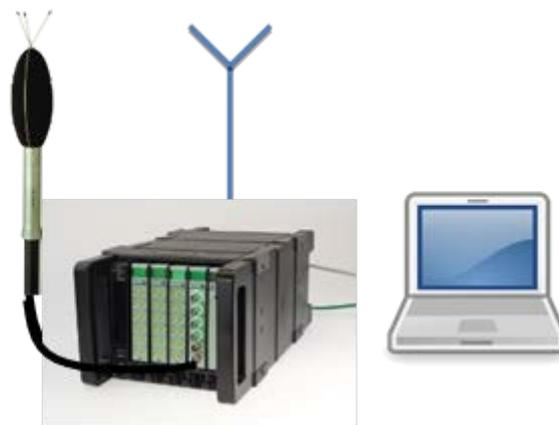
Figure 47: Setup using front-ends for synchronous data, including a GPS antenna for synchronization.
