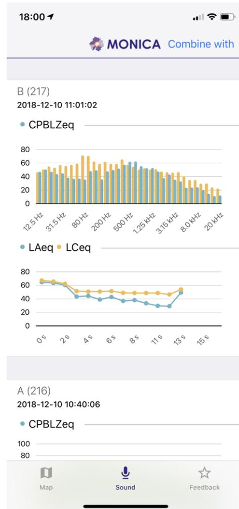
**Figure 24. 1/3 Octave spectra, for SLM B combined with SLM A at Fête des Lumières**
