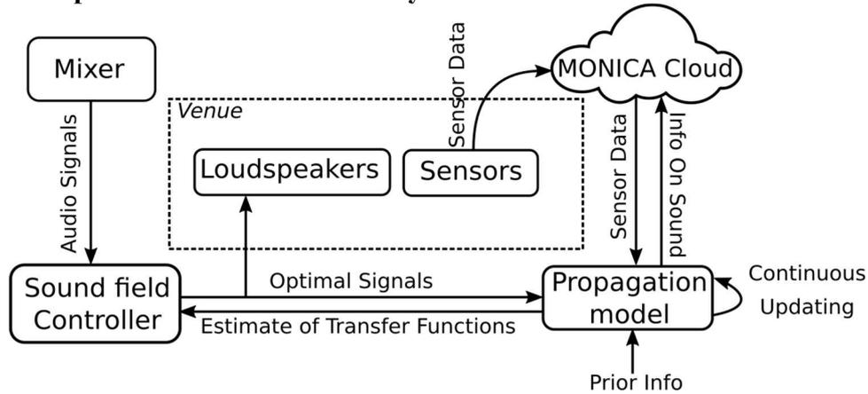
Figure 3: Information flow of MONICA Adaptive Sound Field Controller
