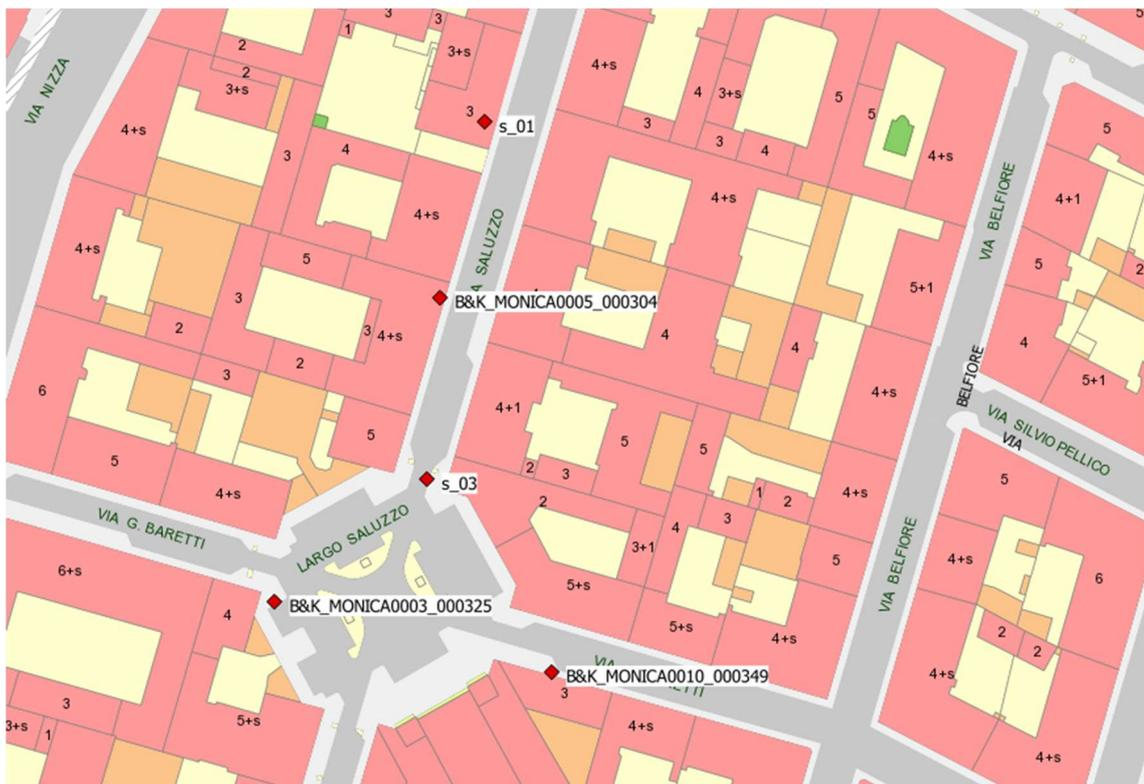
Figure 8: Sound Level Meters deployment during MOVIDA.
