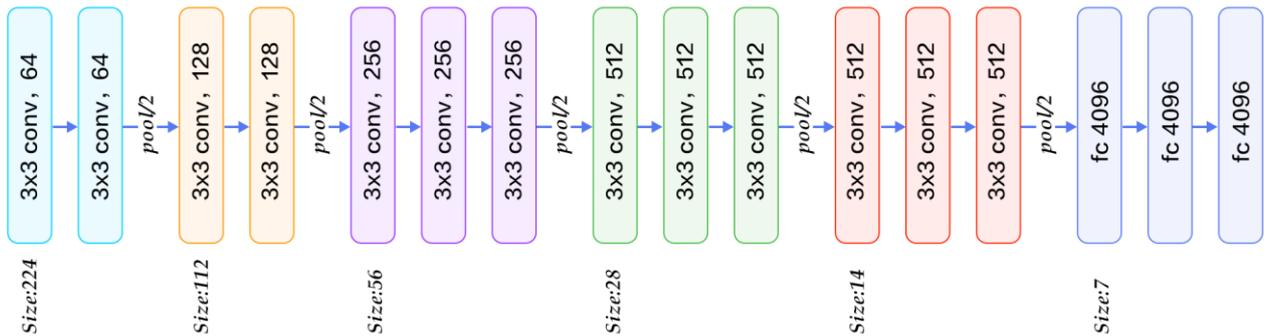
Figure 12: The VGG16 CNN model is used to extract spatial features from each input frame.
