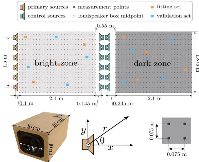
**Figure 30: Setup with 1400 microphones (dots) and 18 loudspeakers. Four microphones in blue were used to fit the model and reconstruct the transfer functions.**
