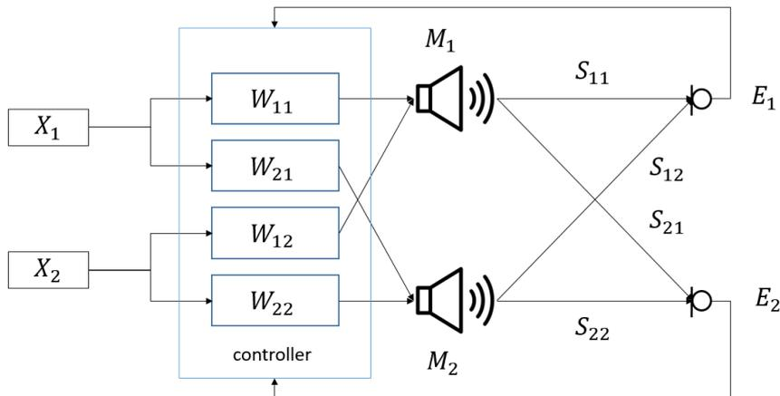
Figure 18: Multichannel Controller Architecture. X: Reference signal (from mixing engineers console),  $W_{ii}$  FIR filters,  $M_i$  Secondary loudspeakers,  $S_{ii}$  sound propagation paths,  $E_i$ : Error measurement positions.
