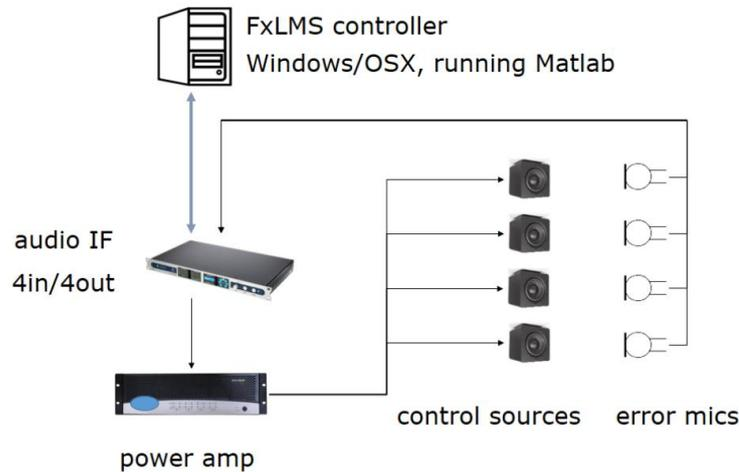
**Figure 19: Technical Architecture of the Quiet Zone system (active part).**
