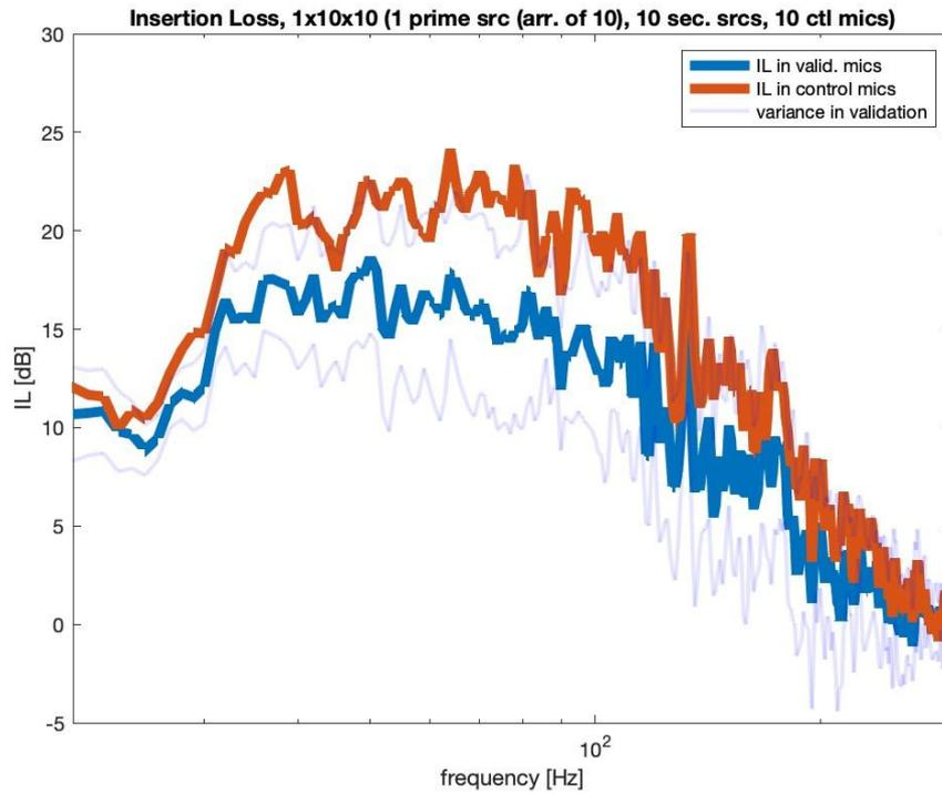
Figure 14: The performance of ASFCs when driven by adaptive QZ algorithm using 10 control microphones
