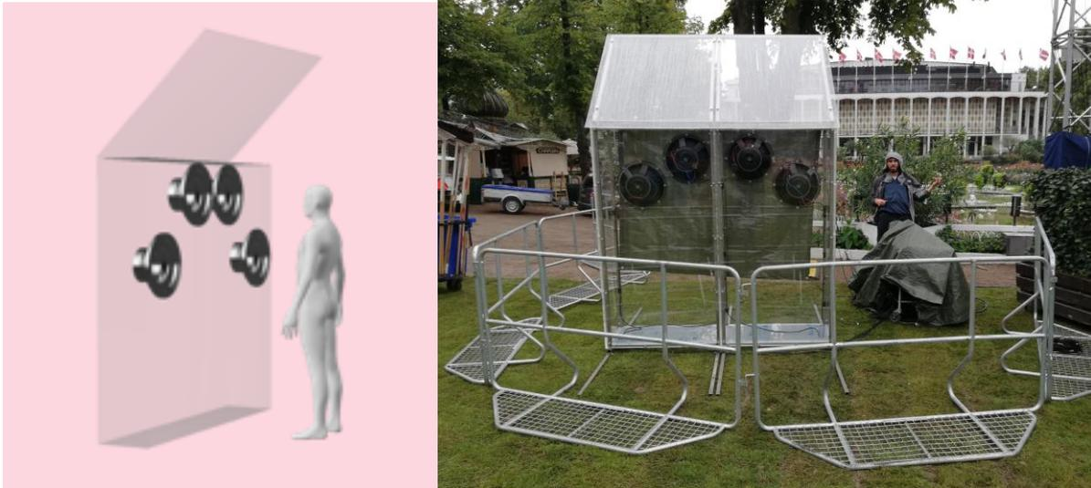
Figure 17: Prototype of the Quiet Zone System tested at the Tivoli pilot site. The controller and the error microphones are not shown here.
