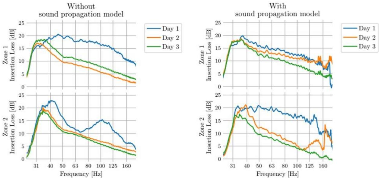
Figure 6: Performance metrics at outdoor experiment. (Top) insertion loss. (Bottom) primary to secondary ratio
