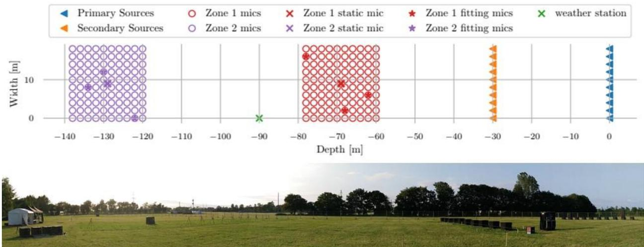
Figure 5: Experimental setup of large scale experiment at Roskilde. Top: Plan of microphones and loudspeakers. Bottom: Photograph of setup.
