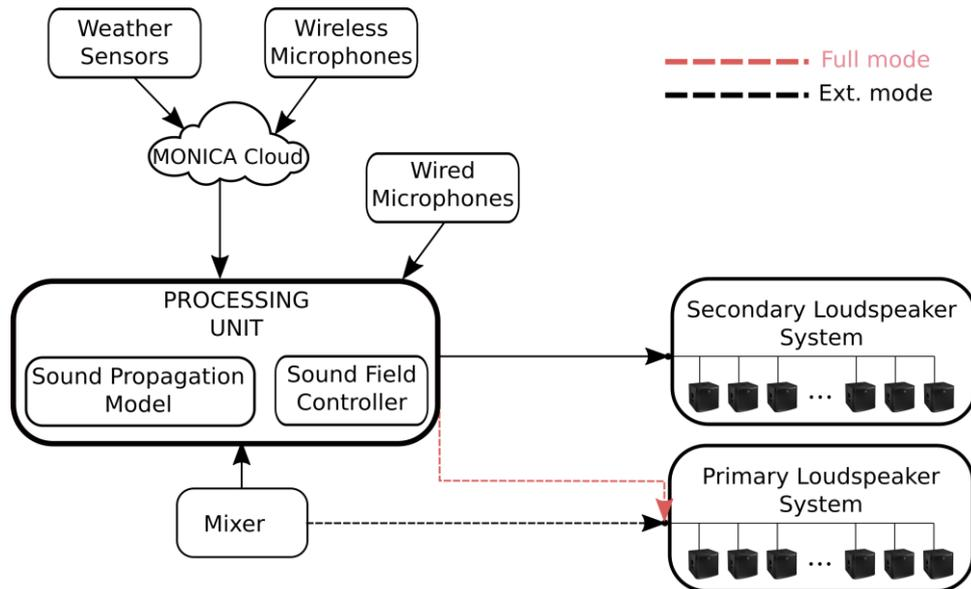
**Figure 3: Infrastructure and deployment of the ASFC. In full mode the primary loudspeaker system is fed from the Processing Unit. In the Extension Mode the primary loudspeaker system is fed directly from the mixer**
