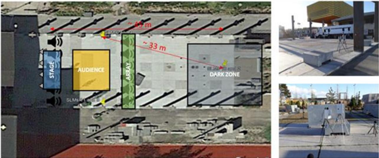
**Figure 33: The Reference SLM is located near the Audience, the remote SLM is placed in the Dark Zone. The top right image shows the reference SLM, Bottom right shows the remote SLM. The SLMs were doubled: one was used for only levels monitoring, the other for audio recordings.**
