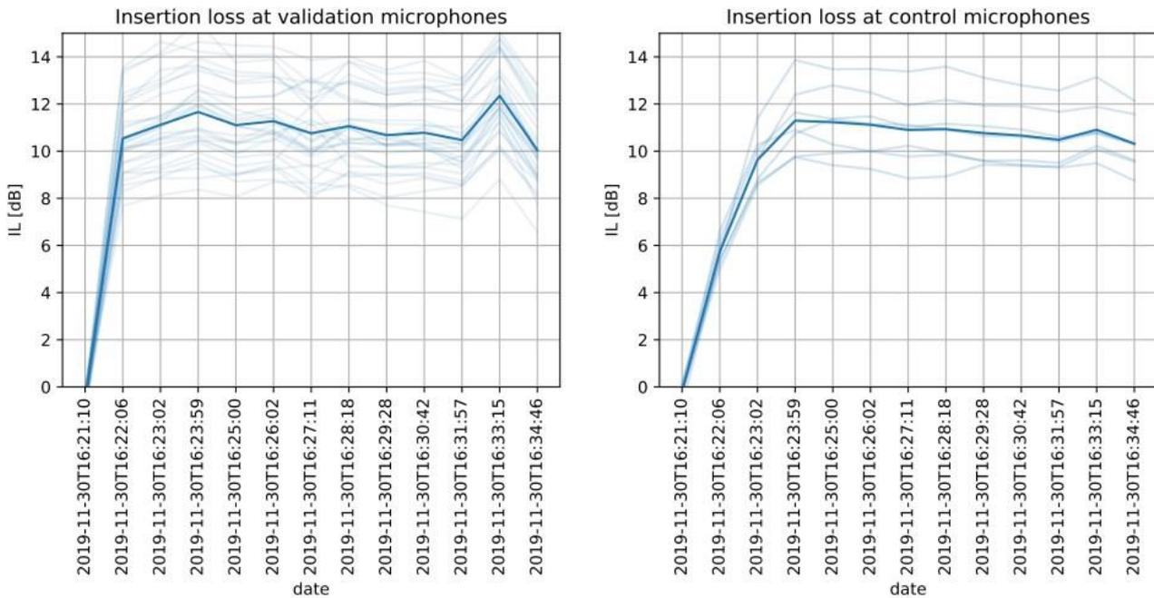
Figure 13: Insertion loss over time averaged over the frequency range 37-110 Hz at validation (left) and control (right) microphones during a 15 minute measurement window at the Sound Summit pilot. Mean over microphones in thick line.
