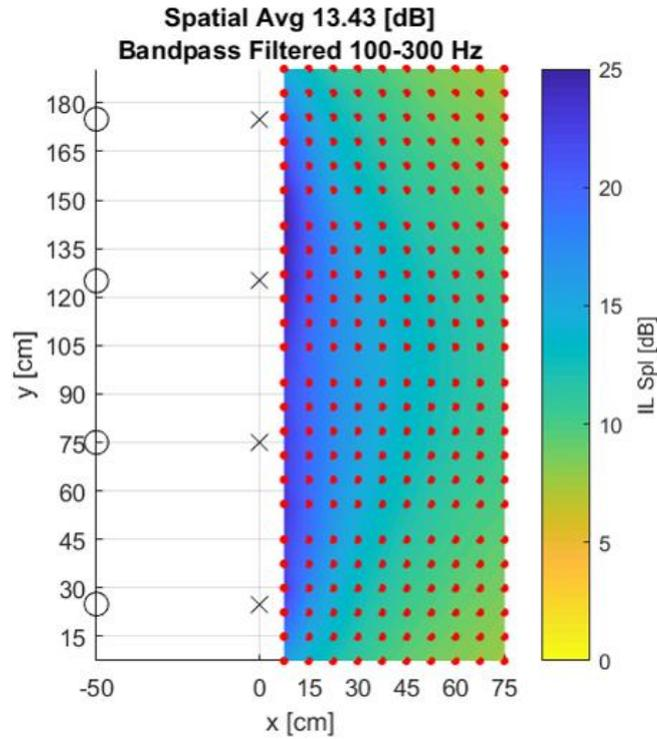
Figure 21: Measured Insertion Loss in Quiet Zone, red dots: measurement positions, black circles: control sources, black crosses: error microphones
