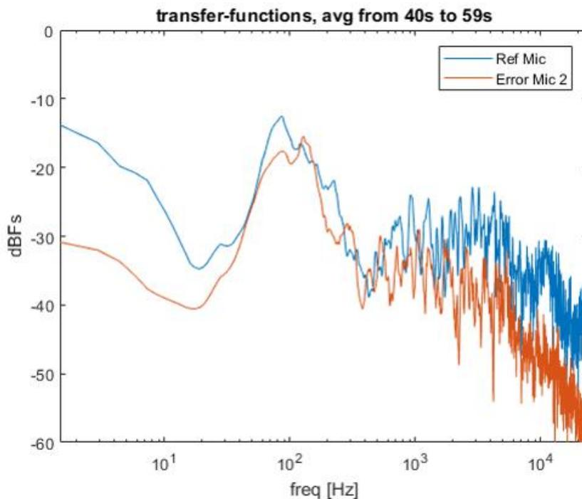
**Figure 23: Extracted transfer functions from an Error Microphone and the Reference Microphone.**
