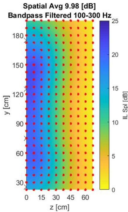
Figure 22: Vertically measured Insertion Loss, up to 10 dB attenuation 30cm above the microphone array
