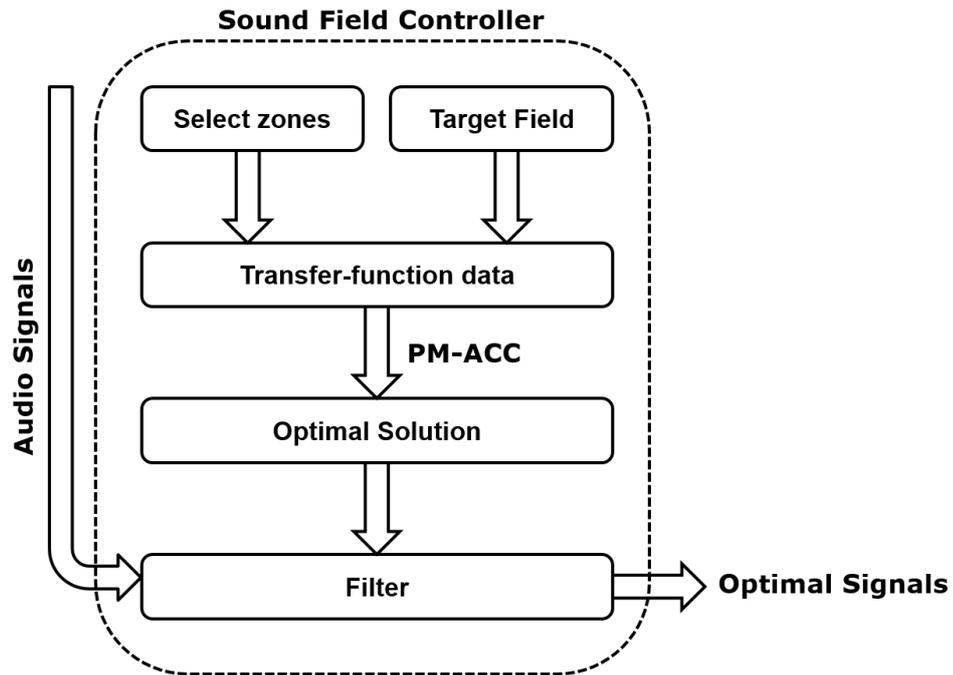
Figure 28: Signal processing flow of the Sound Field Controller, which is a module shown in Figure 2.
