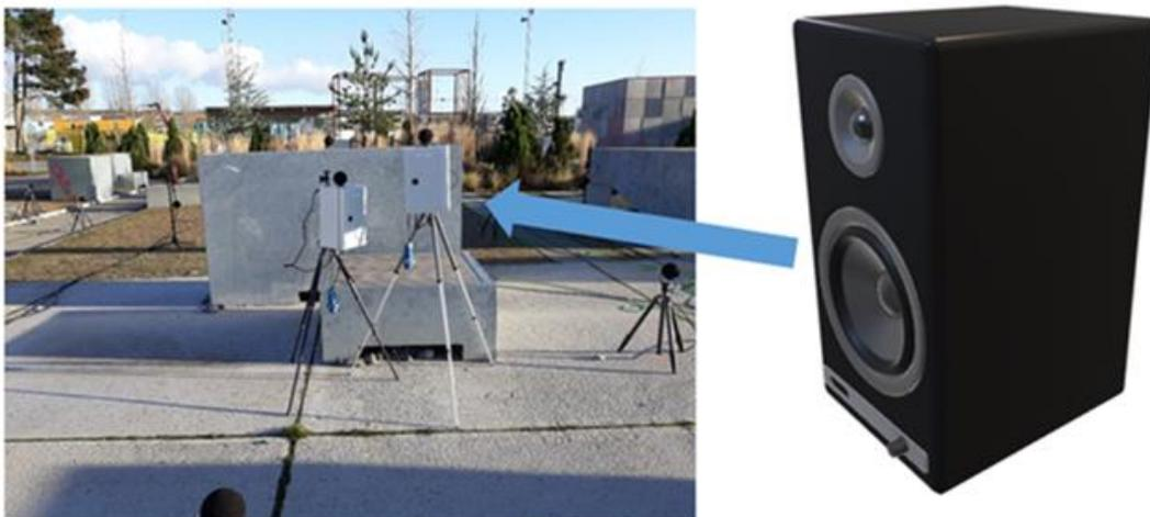
**Figure 34: Loudspeaker nearby the remote SLM, adding an acoustic contribution to the recording.**
