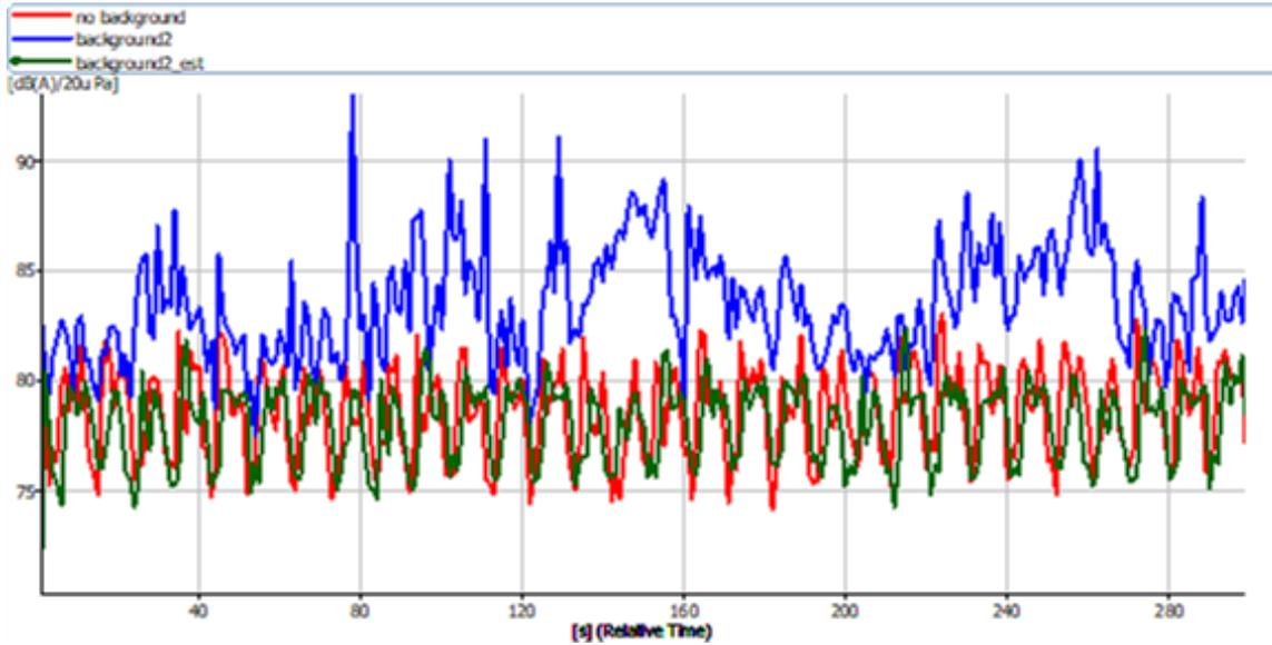
**Figure 35: Validation of Contribution analysis over a 5 minutes window. The blue curve shows the 1 second-LAeq levels as measured by the remote SLM, containing both contributions: from the venue and from the side loudspeaker. The red curve shows the reference LAeq levels, which represent the true contribution that we want to estimate. The green curve shows the LAeq level estimated by the Contribution analysis algorithm.**
