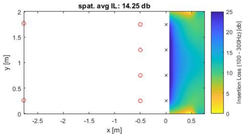
**Figure 20: Results from Simulations.** This plot shows the Insertion loss in the quiet zone (colored area). Red circles on the left: the venue loudspeakers, red circles in the middle: control speakers, black crosses: error microphones. The insertion loss averaged over the whole zone is 14.25 dB.
