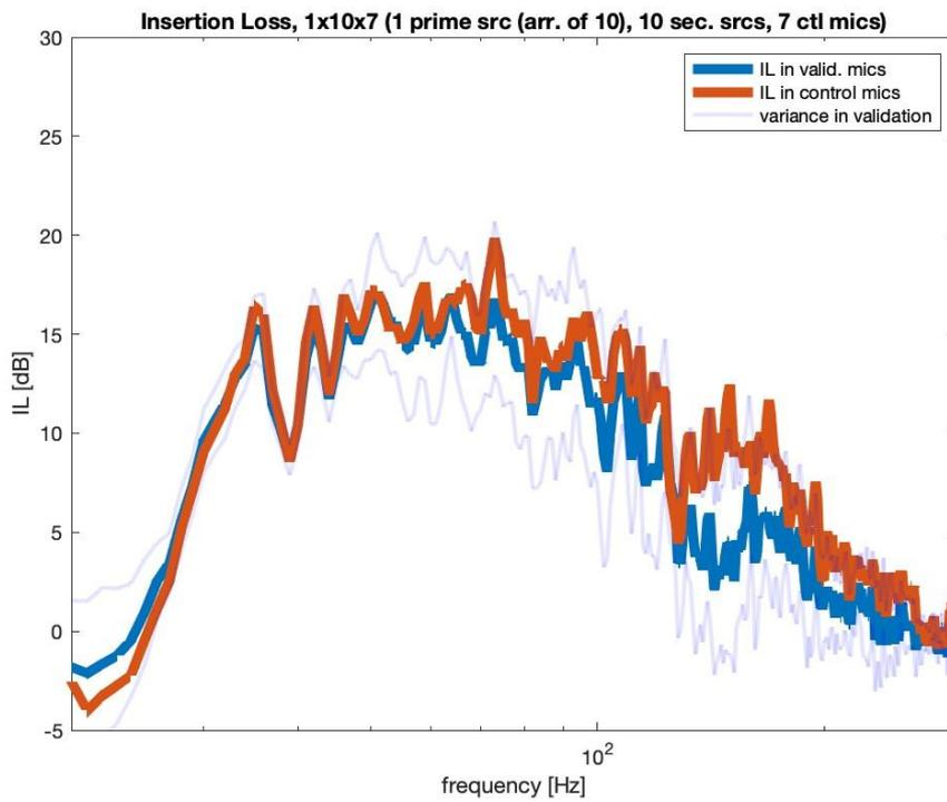
Figure 15: The performance of ASFCs when driven by adaptive QZ algorithm using 7 control microphones
