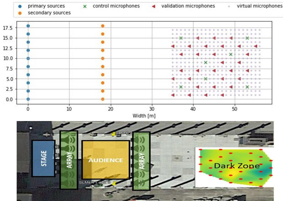
Figure 12: Layout and photo of sound field control setup at Sound Summit 2019
