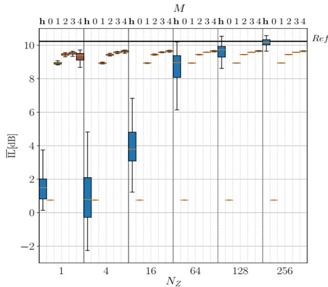
Figure 29: Insertion loss averaged from 100 to 1000 Hz. The box plots show the median in orange and the boxes extend from first to third quartile. The whiskers represent the extreme cases (max and min). Bottom x-axis: Number of measurement positions. Top x-axis: Truncation number in the spherical harmonics basis. h: No model used. Ref: Insertion loss using half of the dense grid of measured transfer functions .
