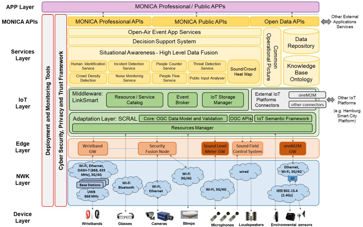
**Figure 2: Functional View of the MONICA Platform Architecture**
