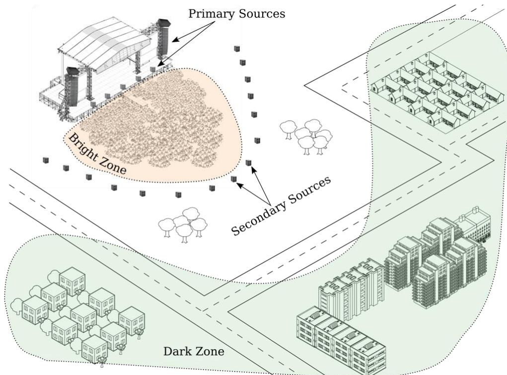
**Figure 36: Basic principle of the MONICA Adaptive Sound Field Control solution**
