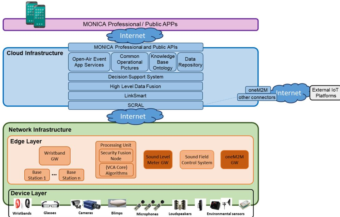
**Figure 3: MONICA High-Level Deployment Architecture**
