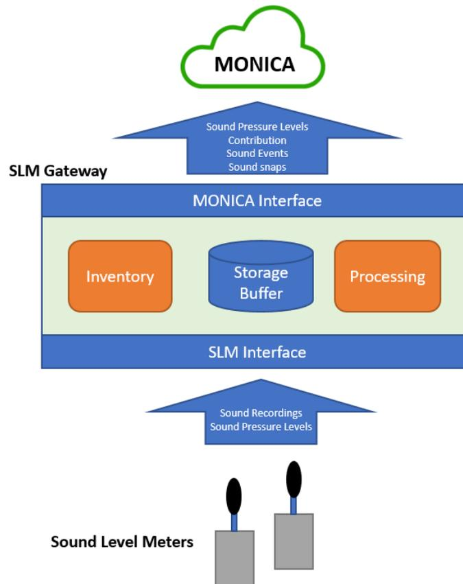
**Figure 30: IoT Sound Level Monitor concept**
