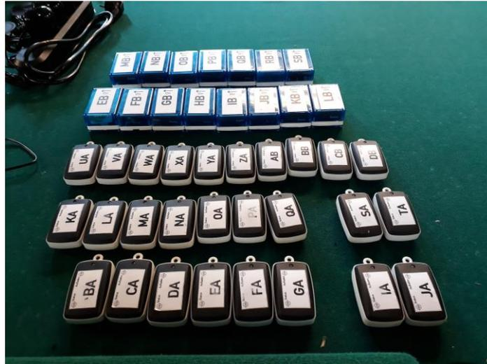
Figure 116: First (top) and second generation of LiPS trackers (bottom)
