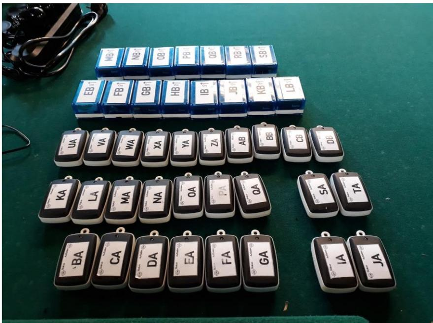
**Figure 79: first iteration prototype (blue) and second iterations prototype (black) of LiPS staff tracker hardware**
