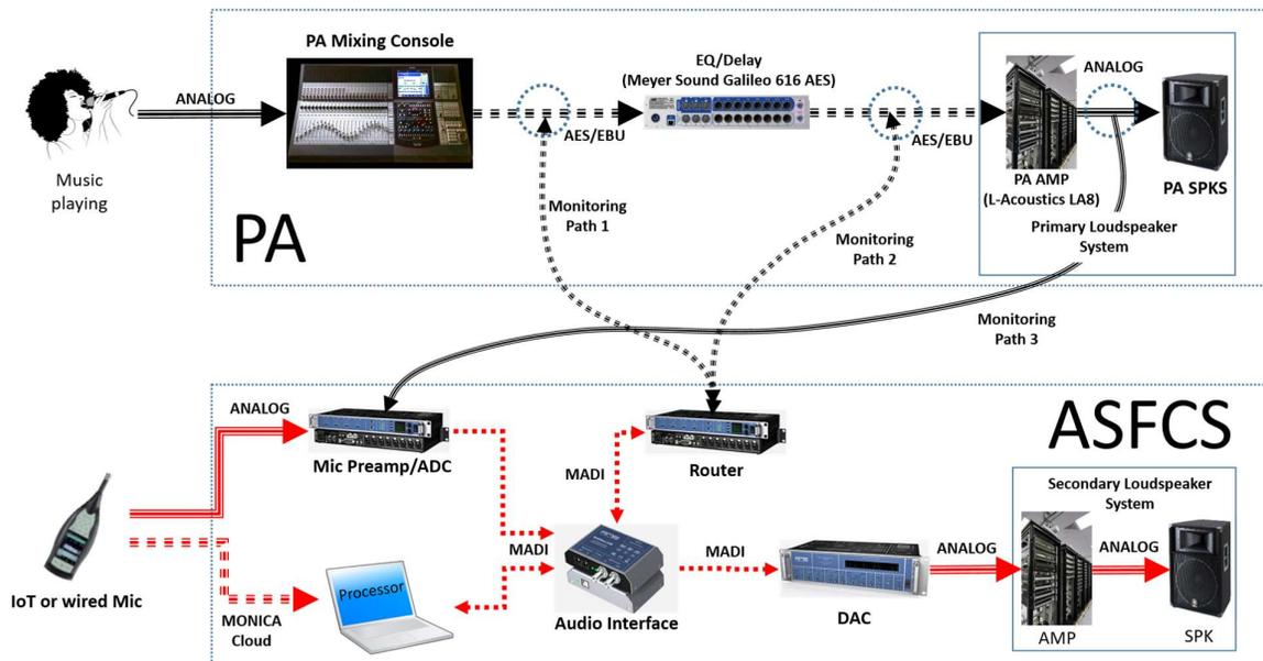
**Figure 4: Example of ASFCS connected with PA system of the pilot at Tivoli**
