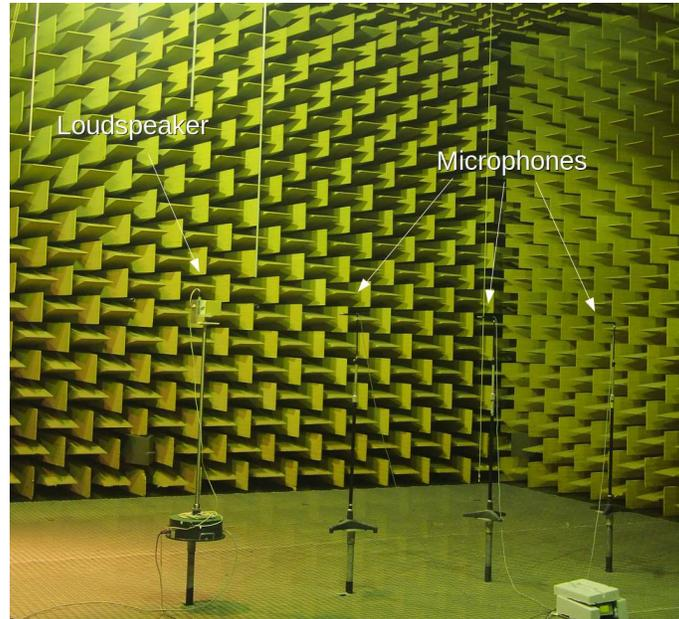
**Figure 10: Measurement setup for loudspeaker characterization**
