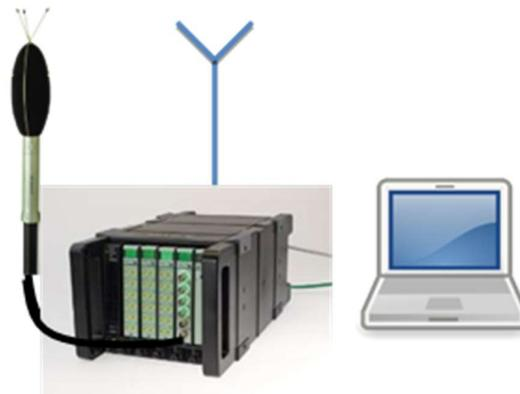
**Figure 21: Setup using front-ends for synchronous data, including a GPS antenna for synchronization.**
