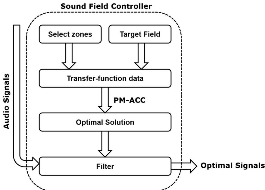
Figure 18: Signal processing flow of the Sound Field Controller, which is a module shown in Figure 2.
