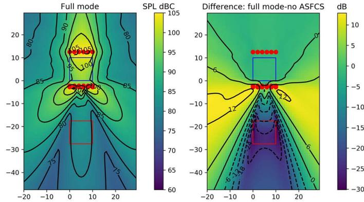
Figure 6: Comparison of total sound pressure level in the vicinity of the simulated venue, small dark zone.<sup>4</sup>
