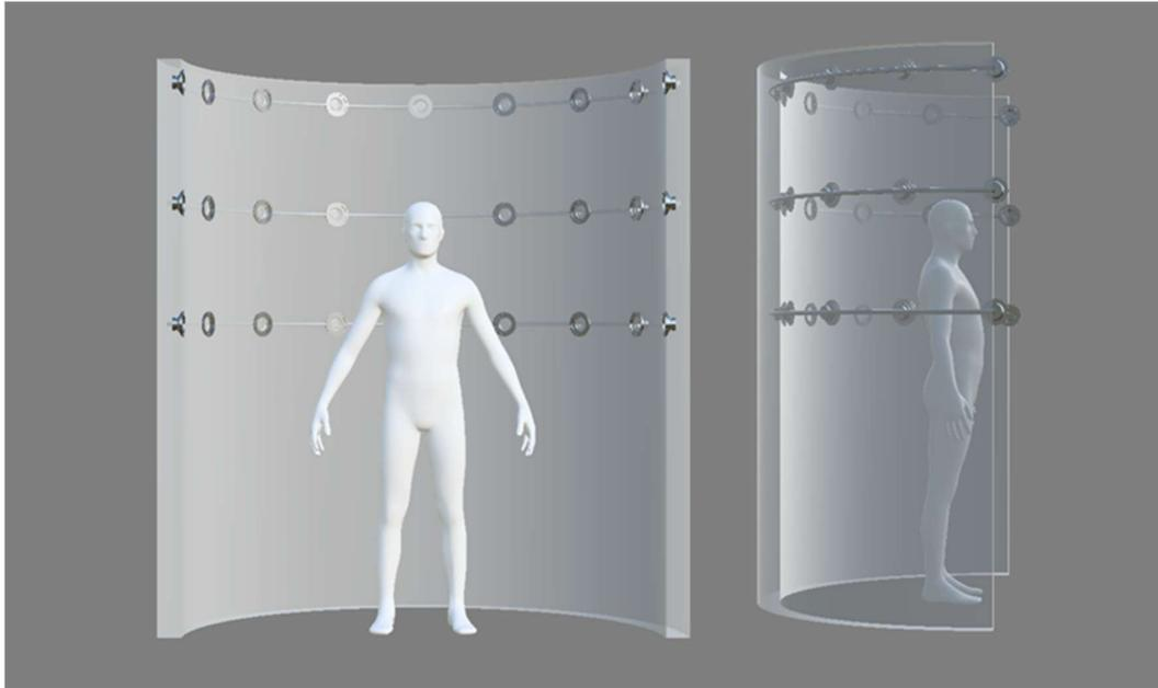
**Figure 13: A possible prototype of a local quiet zone system. Loudspeakers are used to actively attenuate low frequencies, a wall is used to passively reduce high frequencies.**
