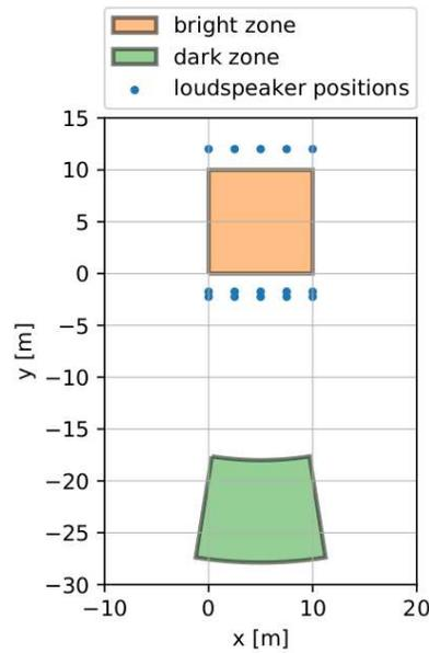
**Figure 19: Setup of bright zone, dark zone and fixed loudspeaker positions in the simulation.**
