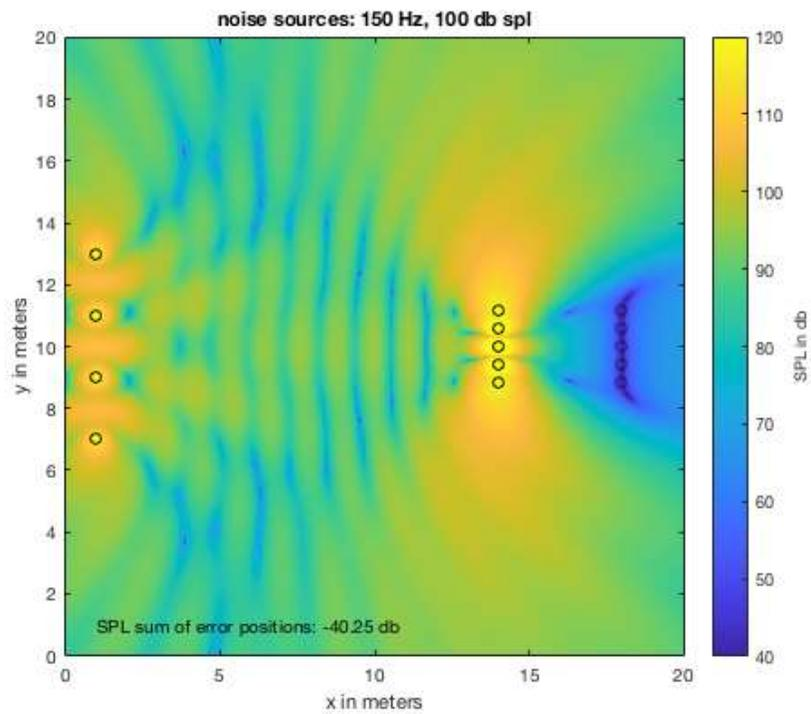
Figure 17: Error Mic positions further away from the control sources. It is obvious how the control sources contaminate the surrounding.
