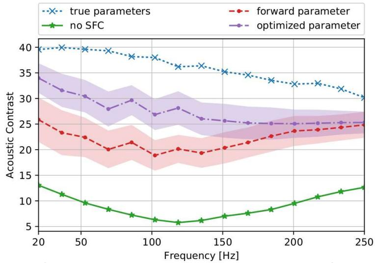
**Figure 20: Comparison of acoustic contrast when using true parameters (blue), forward parameters (red), optimized parameter with Bayesian inference (purple) and no SFC (green).**
