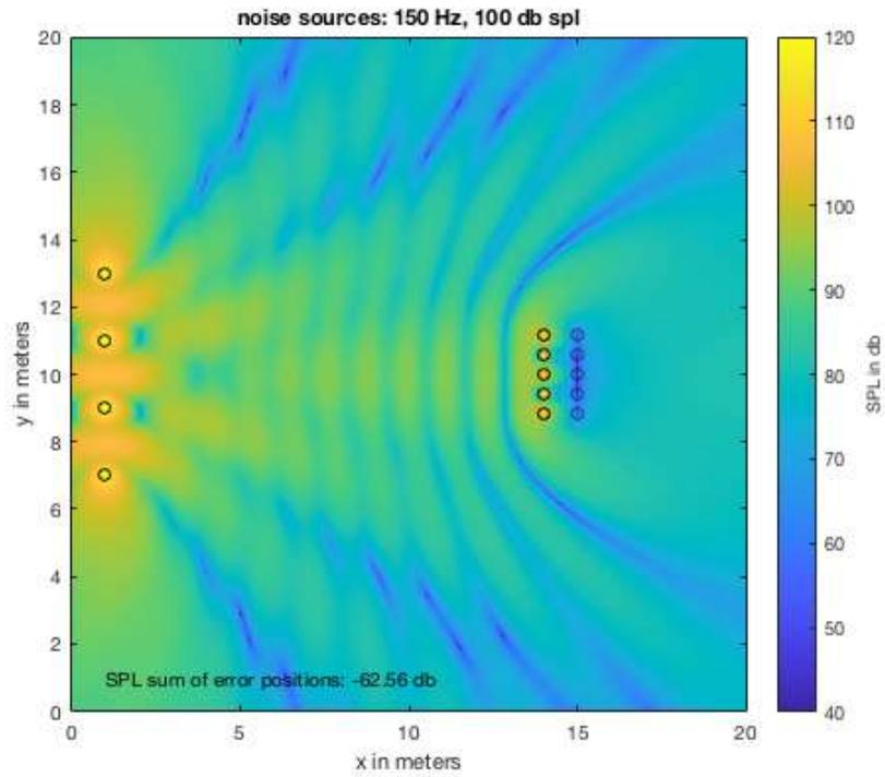
Figure 16: Error Mic positions close to the control sources with a distance of 0.5m in between. Note that at 150 Hz this distance is smaller than a quarter of a wavelength.
