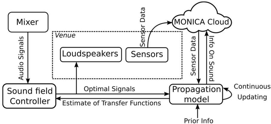
**Figure 2: Information flow in the sound field control system**
