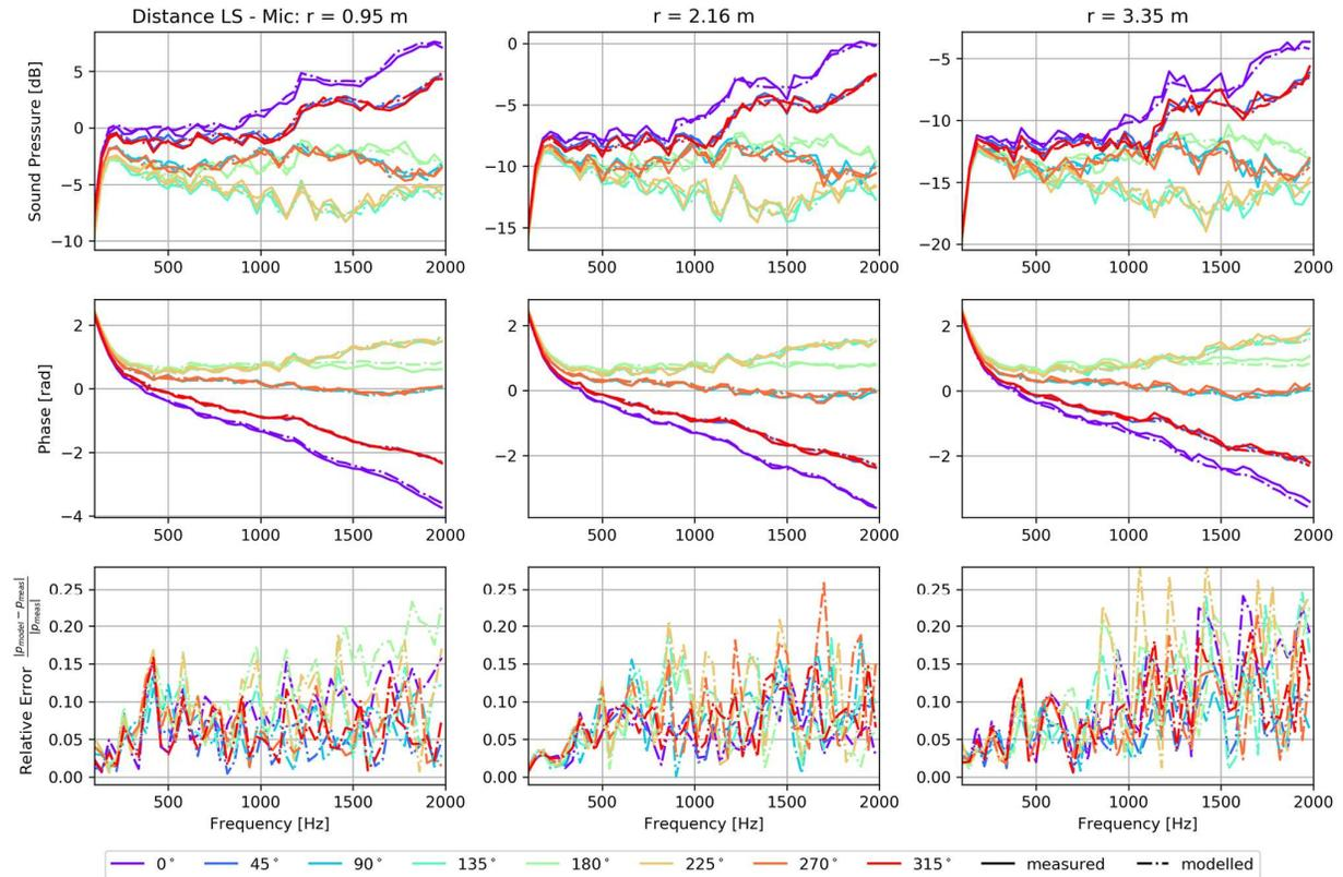
**Figure 11: Modelled and measured response of the loudspeaker under test at the microphone positions together with the relative error. Note that the phase is back-propagated in time and unwrapped for a clearer presentation and readability.**
