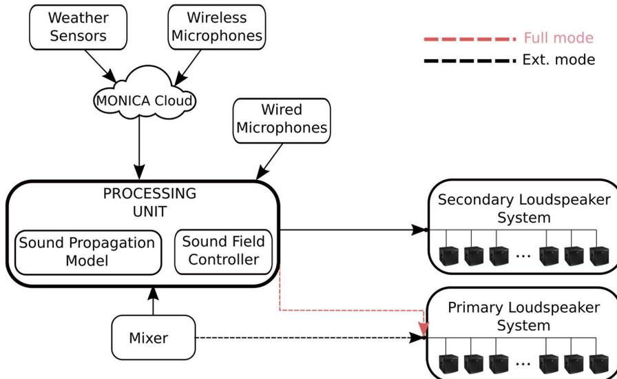
**Figure 3: Infrastructure and deployment of the ASFCS. In full mode the primary loudspeaker system is fed from the Processing Unit. In the Extension Mode the primary loudspeaker system is fed directly from the mixer**
