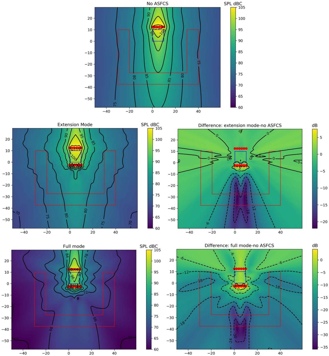
Figure 8: Comparison of total sound pressure level in the vicinity of the simulated venue, surrounding dark zone
