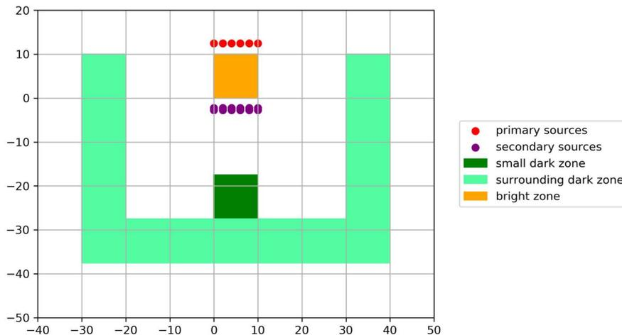
**Figure 5: Sketch of the adaptive sound field control system, which is optimized for a good audio experience in the bright zone and low sound pressure level in the dark zone**
