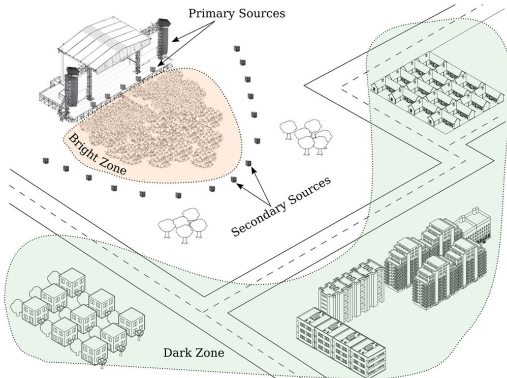
**Figure 1: Sketch of the adaptive sound field control system, which is optimized for a good audio experience in the bright zone and low sound pressure level in the dark zone**
