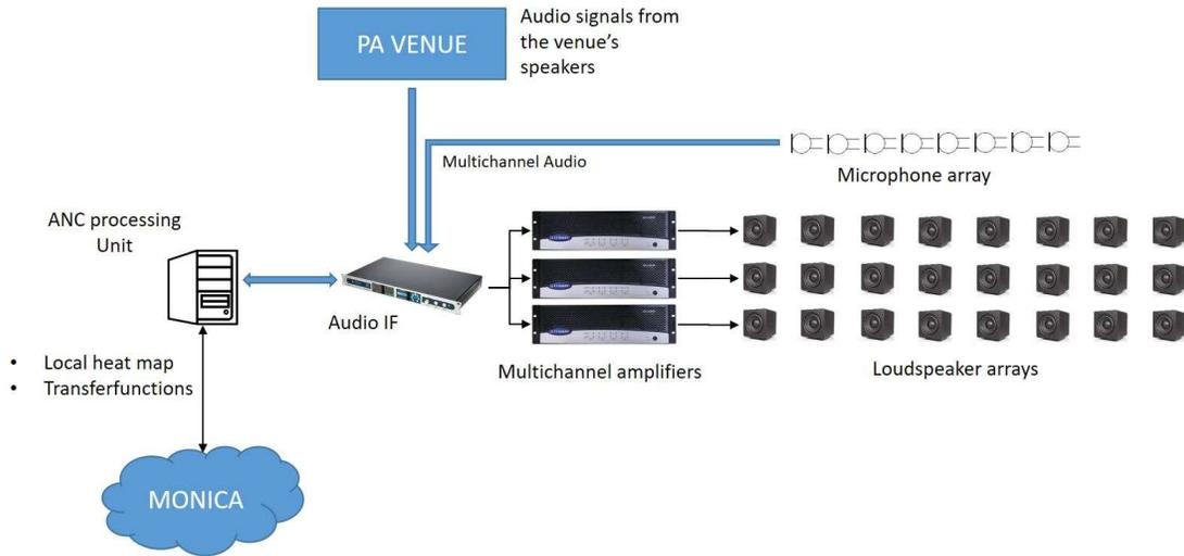
**Figure 14: The components of the active part of the quiet zone system**
