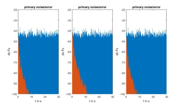
Figure 9: This figure shows the noise signal (blue) at three error microphone positions. The red signal is the total pressure at the error mics. It can be seen how the adaptive filter comes in and reduces the total pressure over time.
