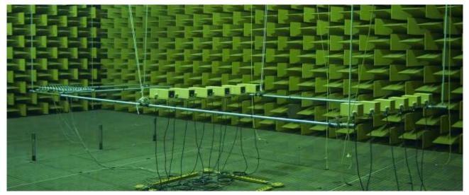
Figure 1: Laboratory experiment of the sound field control system in DTU's anechoic chamber
