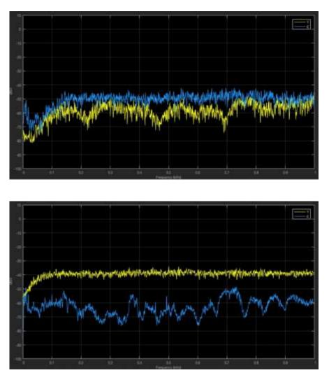
Figure 8: This figure shows the noise signal (blue) and the controller signal (yellow). TOP: The adaptive filter hasn't converged yet, the noise signal looks like without active control (around -50db). BOTTOM: The adaptive filter has converged/reached steady state and the noise signal is attenuated up to 20db (-50db -> -70db).
