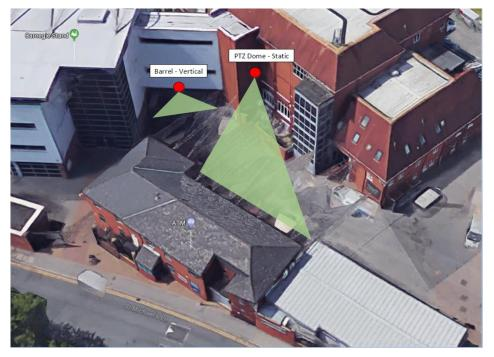
Figure 63. Camera to be mounted on the walkway above
