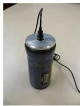
Figure 20. Kit for external installation and calibration of Lavalier microphone with a Class 1 source.
