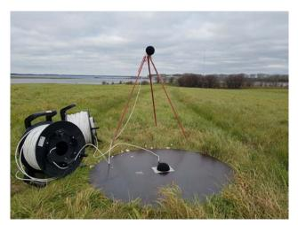
Figure 39: Microphone arrangement in pairs for each of the recording points
