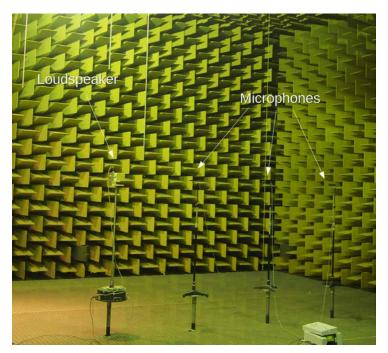
Figure 10: Measurement setup for loudspeaker characterization
