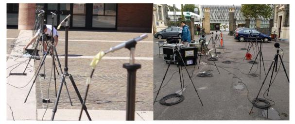
Figure 49: Non-wired measurements of Transfer Functions at KFF2018 (Left) and Tivoli 2018 (Right). An array of 10 microphones where connected to a B&K frontend equipped with GPS time synchronization.
