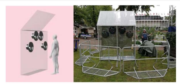
Figure 24: Prototype of the Quiet Zone System tested at the Tivoli pilot site. The controller and the error microphones are not shown here.
