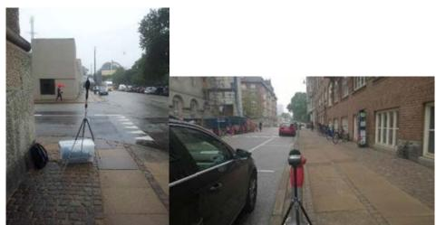
Figure 48: Measurements outside Tivoli 2017 using a front-end (left) and a SLM (right)
