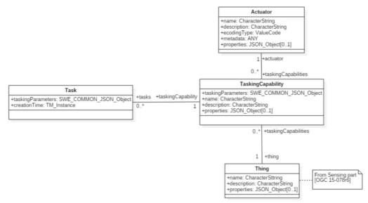
Figure 3 OGC Sensor things API Tasking Model
