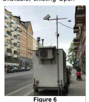
Example of a fixed sensor station for air quality
