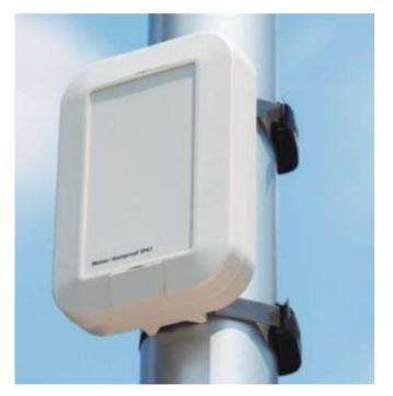
Figure 8 the pole-mounted UWB anchor (Base Station)
