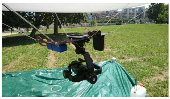
Figure 17: The payload of battery, stabilized camera and sensor array
