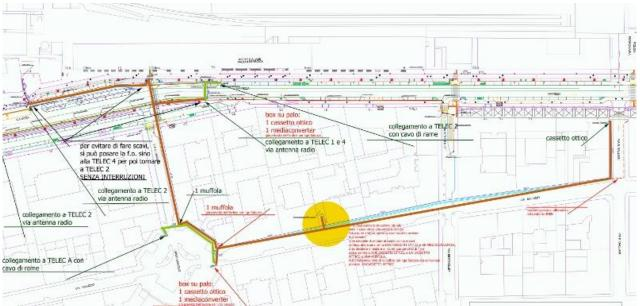
Figure 90: Blueprint of the new glass fiber connection for cameras in Largo Saluzzo, via Saluzzo and via Nizza.
