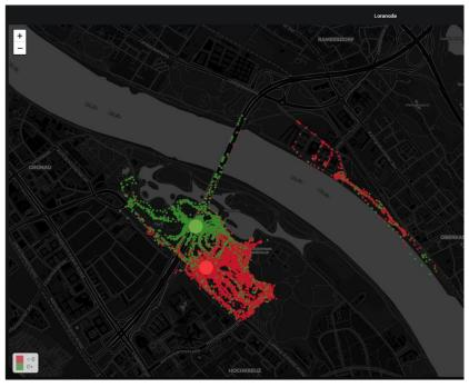
Figure 81: LoRa range of LiPS trackers during Rhein in Flammen 2019
