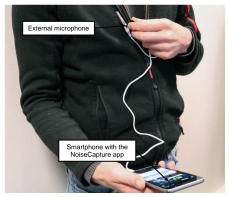
Figure 51: Measurement equipment of a NoiseCapture Party goer
