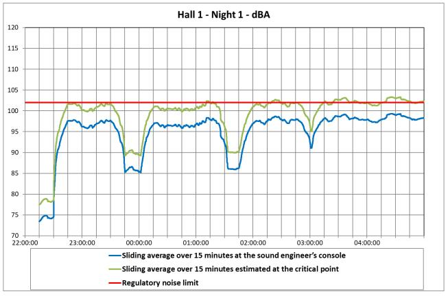
Figure 13: Sound levels fluctuation regarding the regulatory noise limit during the first night
