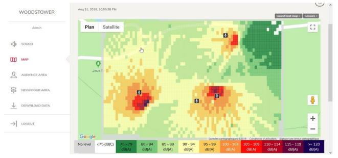
Figure 39: Display of the Sound Heat Map on the COP
