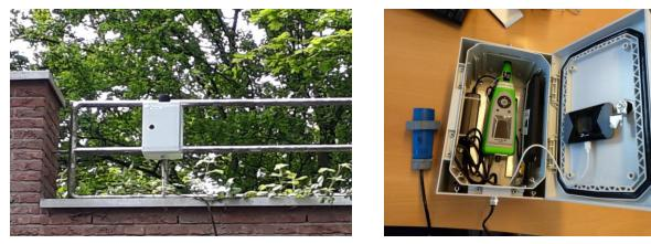
Figure 72: Installed sound level meter
