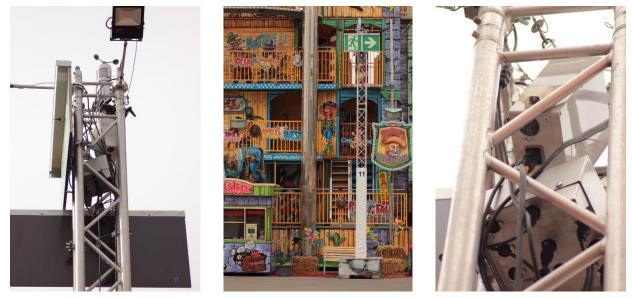
Figure 101: Deployment of environmental sensors with wind speed meters
