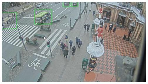
Figure 23: Video analytics algorithm identifying a car
