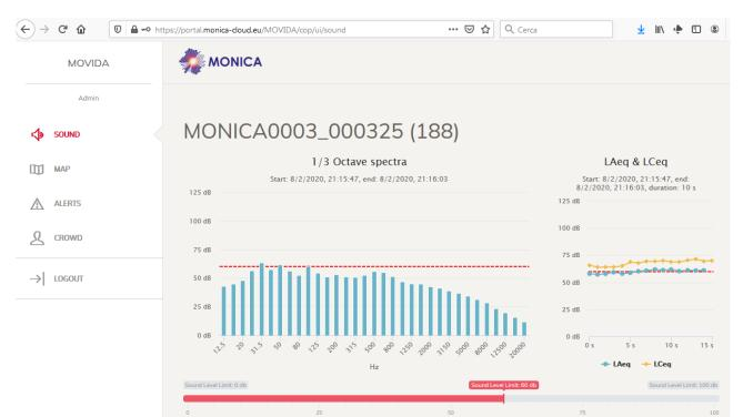
Figure 85: Screenshot of Movida Permanent COP, noise data from Class 1 B&K SLM
