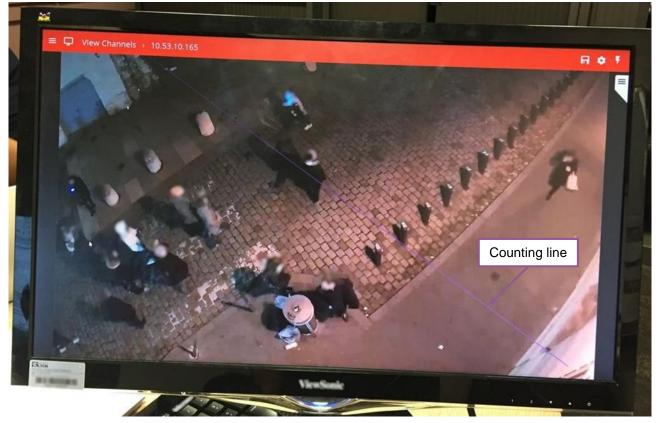
Figure 55: Counting algorithm working on Camera Nr. 5
