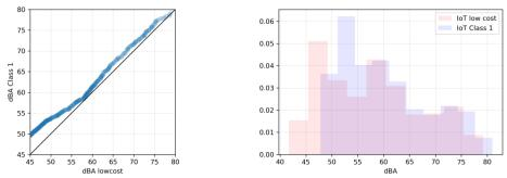
Figure 87: Scatter plot (left) and distribution (right) of hour noise levels in Largo Saluzzo, low-cost vs class 1
