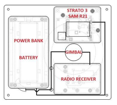
Figure 121: Payload board layout
