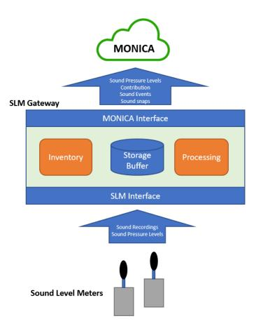
Figure 30: IoT Sound Level Monitor concept
