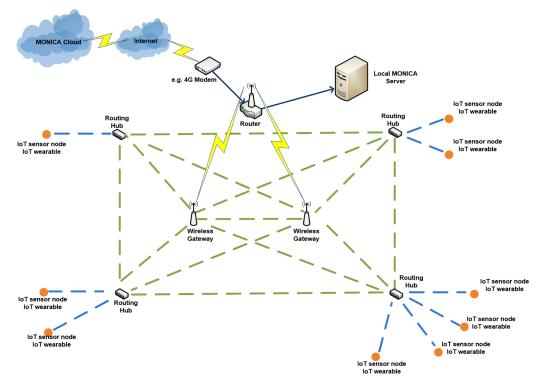
Figure 4: Generic View of the Overall Network Infrastructure Deployment
