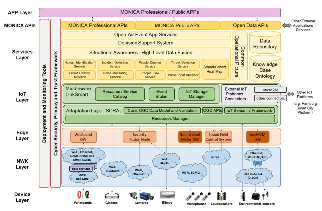
Figure 2: Functional View of the MONICA Platform Architecture
