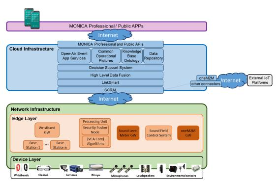
Figure 3: MONICA High-Level Deployment Architecture
