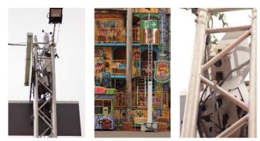
Figure 23: Deployment of environmental sensors with wind speed meter
