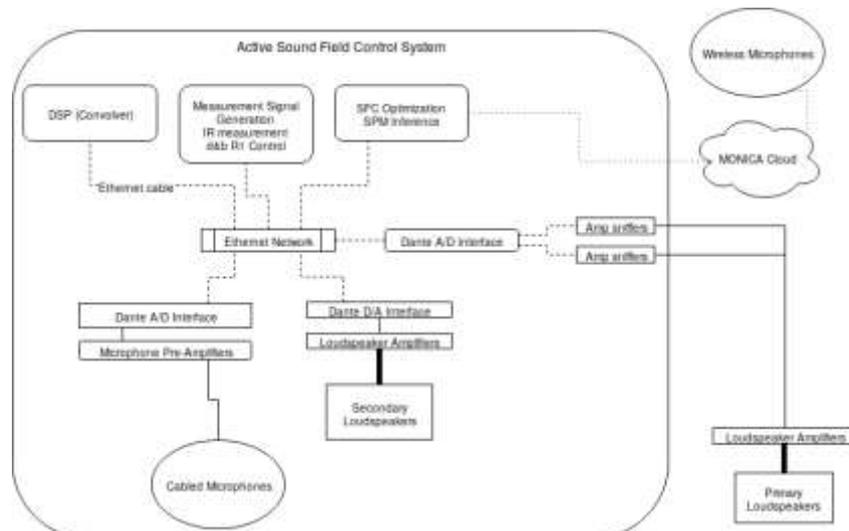
**Figure 13: Wiring scheme of the ASFC deployment at Kappa Futur Festival 2018**
