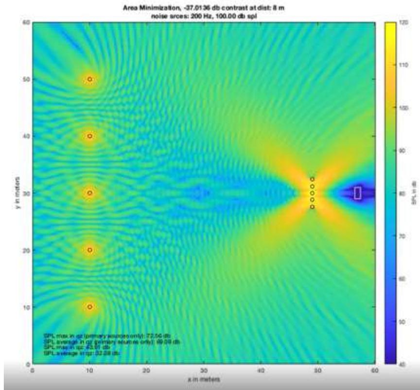
**Figure 6: this figure shows how the output power of the secondary sources increases with distance to the quiet zone. In order to produce the maximum of attenuation in the quiet zone at 8m distance the secondary sources have to produce very high sound pressure levels which radiate into the environment.**
