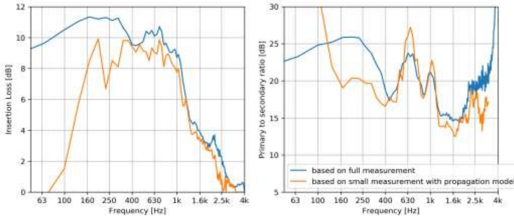
Figure 2: Comparison of performance of sound field control system based on transfer-functions that were directly measured or estimated by the sound propagation model.
