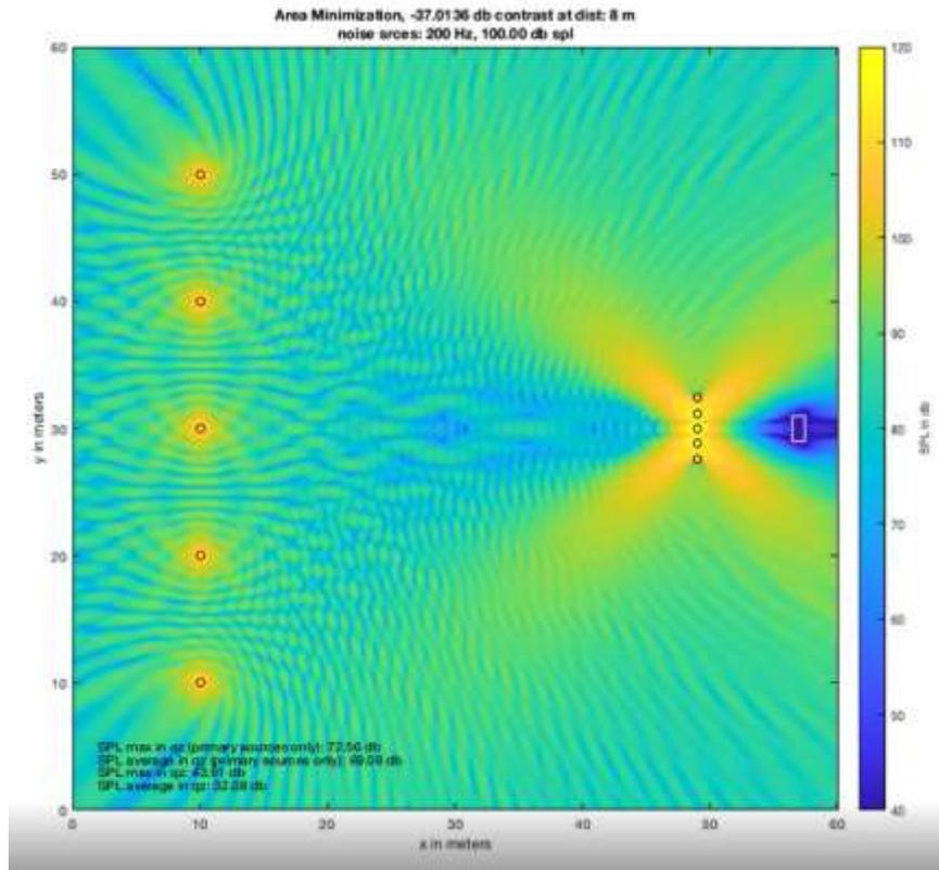
**Figure 6: this figure shows how the output power of the secondary sources increases with distance to the quiet zone. In order to produce the maximum of attenuation in the quiet zone at 8m distance the secondary sources have to produce very high sound pressure levels which radiate into the environment.**
