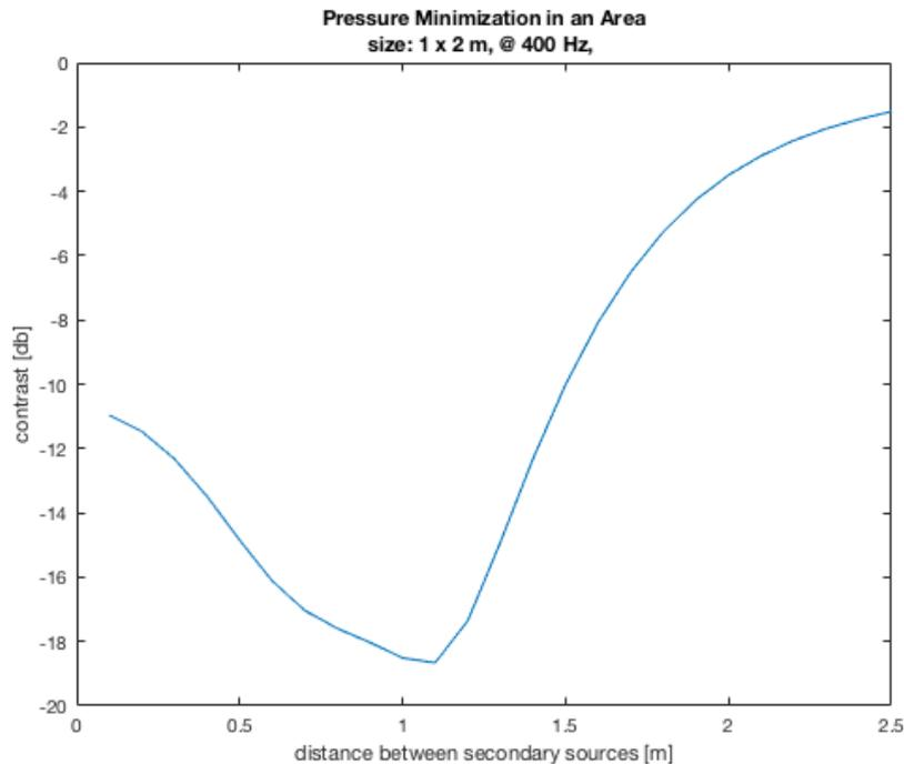
**Figure 7: the amount of attenuation is shown in dependence of the distance in between the secondary loud speakers. For a series of frequencies this dependency has been plotted and it seems that there is an optimal distance of 1-1.2m secondary source distance for frequencies up to 500 Hz.**
