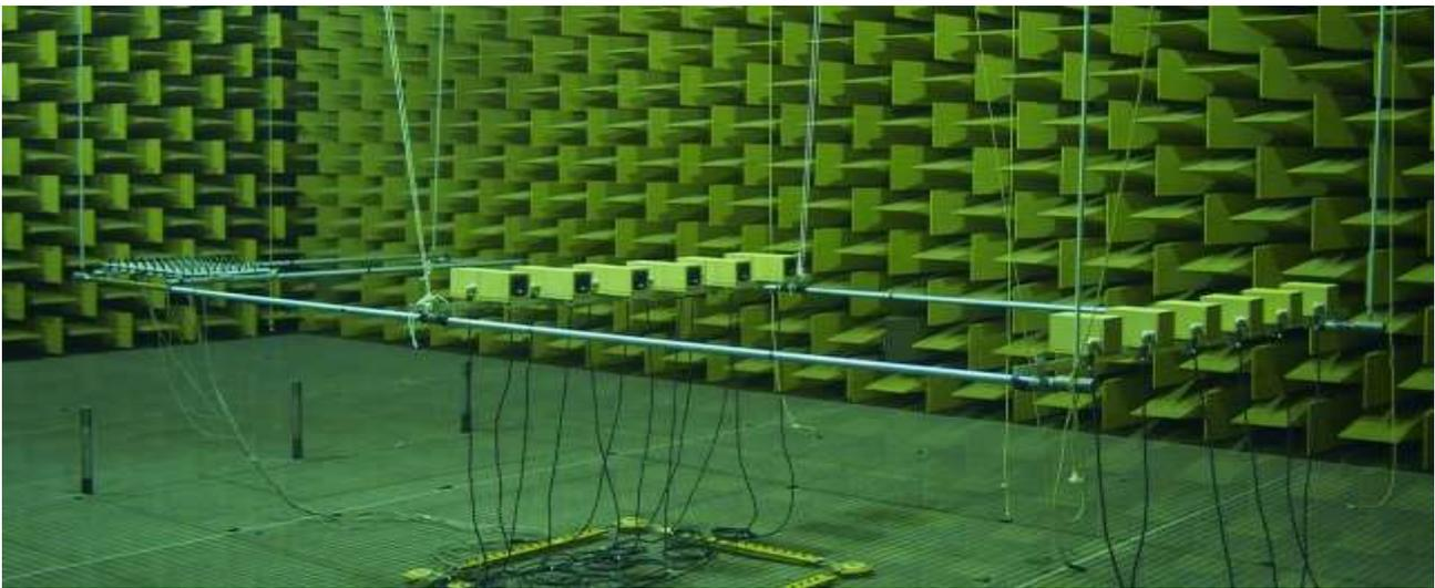
Figure 1: Laboratory experiment of the sound field control system in DTU's anechoic chamber
