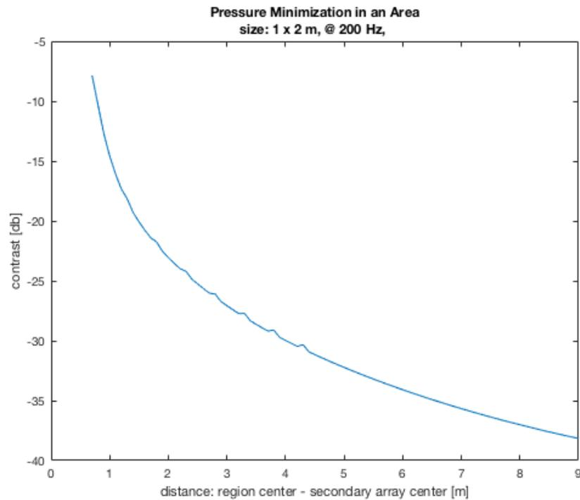
**Figure 5: the maximum amount of attenuation of noise increases with the distance in between the secondary array and the quiet zone. The figure shows the amount of attenuation achieved in average in a 1x2m zone of quiet and by using five secondary sources. (contrast: SPLtotal average in QZ – SPLnoise average in QZ)**
