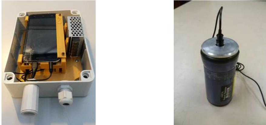
**Figure 20. Kit for external installation and calibration of Lavalier microphone with a Class 1 source.**
