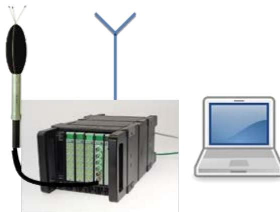
Figure 47: Setup using front-ends for synchronous data, including a GPS antenna for synchronization.
