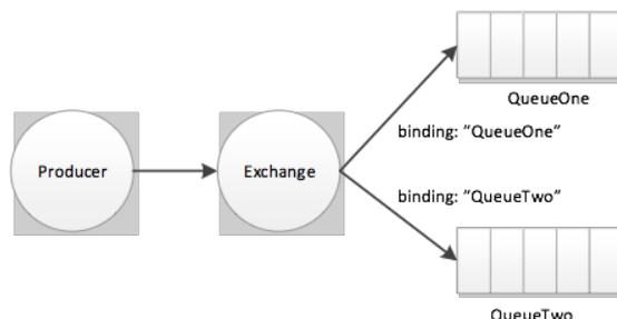
**Figure 12 Direct exchange**
