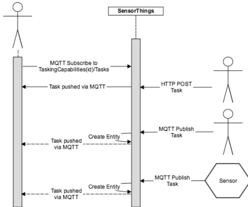
**Figure 4 Listening to Task entities using MQTT**
