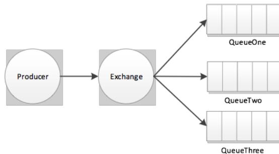
**Figure 13 Fanout exchange**
