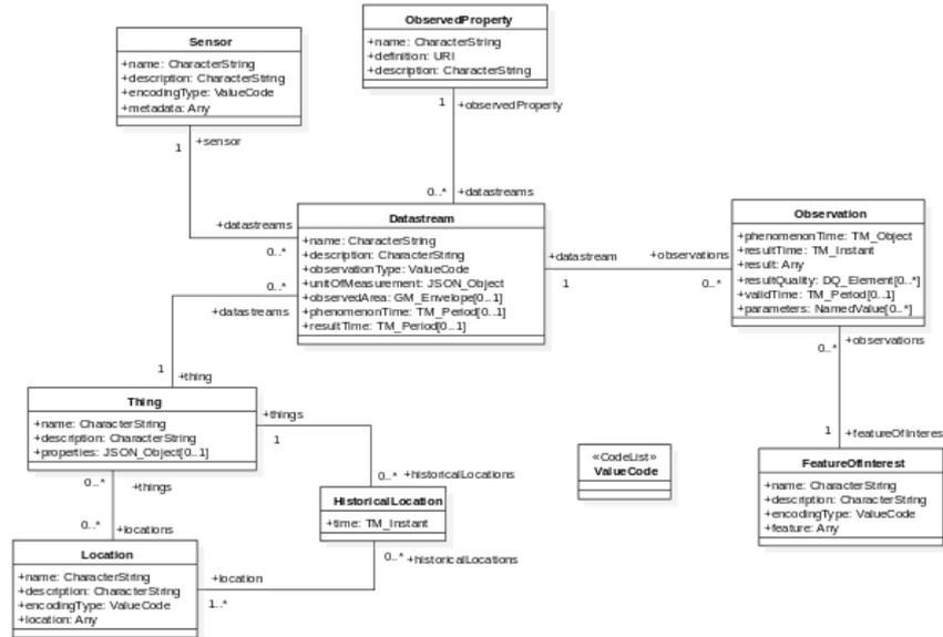
Figure 1 The OGC SensorThings Data Model
