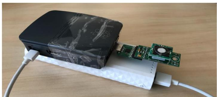
**Figure 4 The mobile sensor gateway for sensing sound levels and air quality parameters**
