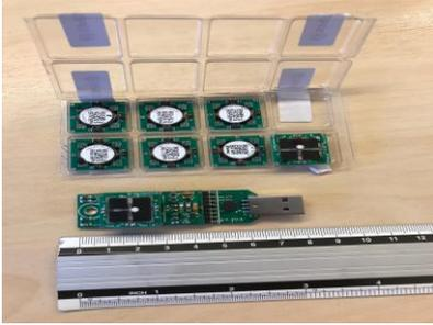
**Figure 5** Examples of sensors that can be attached to the mobile sensor gateway
