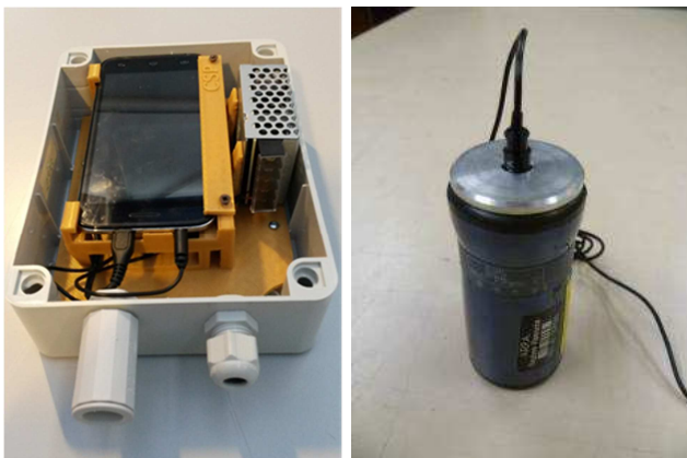
Figure 2. Kit for external installation and calibration of Lavalier microphone with a Class 1 source.
