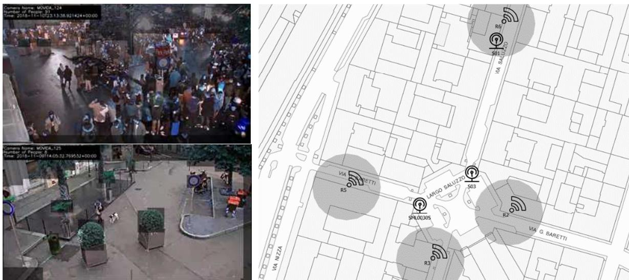
Figure 1: Largo Saluzzo in late night and early morning (left); installed SLMs and WiFi scanner (right)
