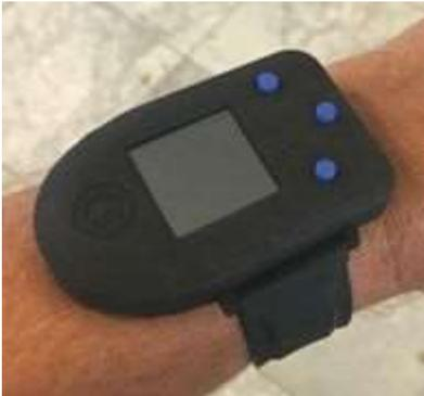
**Figure 6 the UWB Tracking Device for the MONICA Service Staff**
