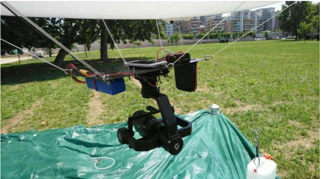
**Figure 17: The payload of battery, stabilized camera and sensor array**
