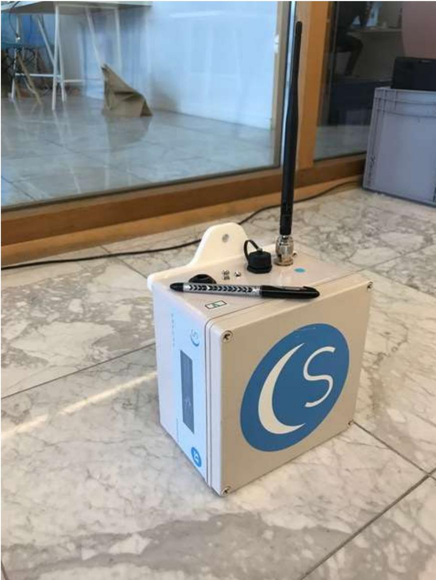
Figure 2 The Sendrato SB1 networked Base Station
