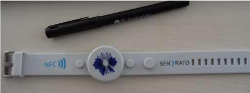
Figure 1 The SENDRATO 800 MHz wristband
