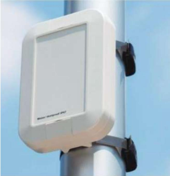
**Figure 8 the pole-mounted UWB anchor (Base Station)**
