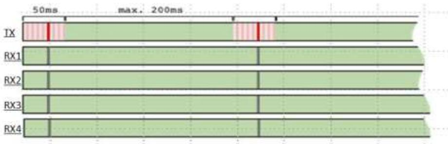
Figure 5 Parallel channel structure (group polling) for a large number of IoT wearables
