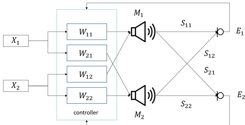
**Figure 18: Multichannel Controller Architecture. X: Reference signal (from mixing engineers console),  $W_{ii}$  FIR filters,  $M_i$  Secondary loudspeakers,  $S_{ii}$  sound propagation paths,  $E_i$ : Error measurement positions.**
