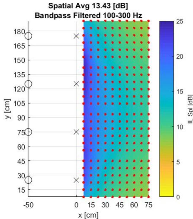
**Figure 21: Measured Insertion Loss in Quiet Zone, red dots: measurement positions, black circles: control sources, black crosses: error microphones**
