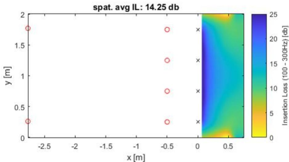
**Figure 20: Results from Simulations.** This plot shows the Insertion loss in the quiet zone (colored area). Red circles on the left: the venue loudspeakers, red circles in the middle: control speakers, black crosses: error microphones. The insertion los averaged over the whole zone is 14.25 dB.
