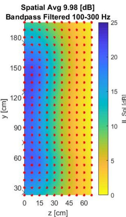
**Figure 22: Vertically measured Insertion Loss, up to 10 dB attenuation 30cm above the microphone array**
