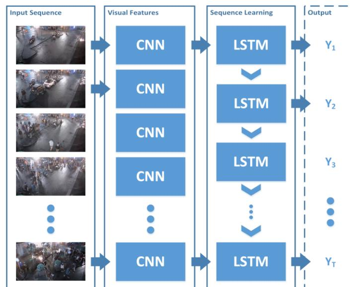
**Figure 8: Long-term Recurrent Convolutional Networks (LRCNs) architecture, leverages the strengths of rapid progress in CNNs for visual recognition is video sequence with time-varying inputs.**
