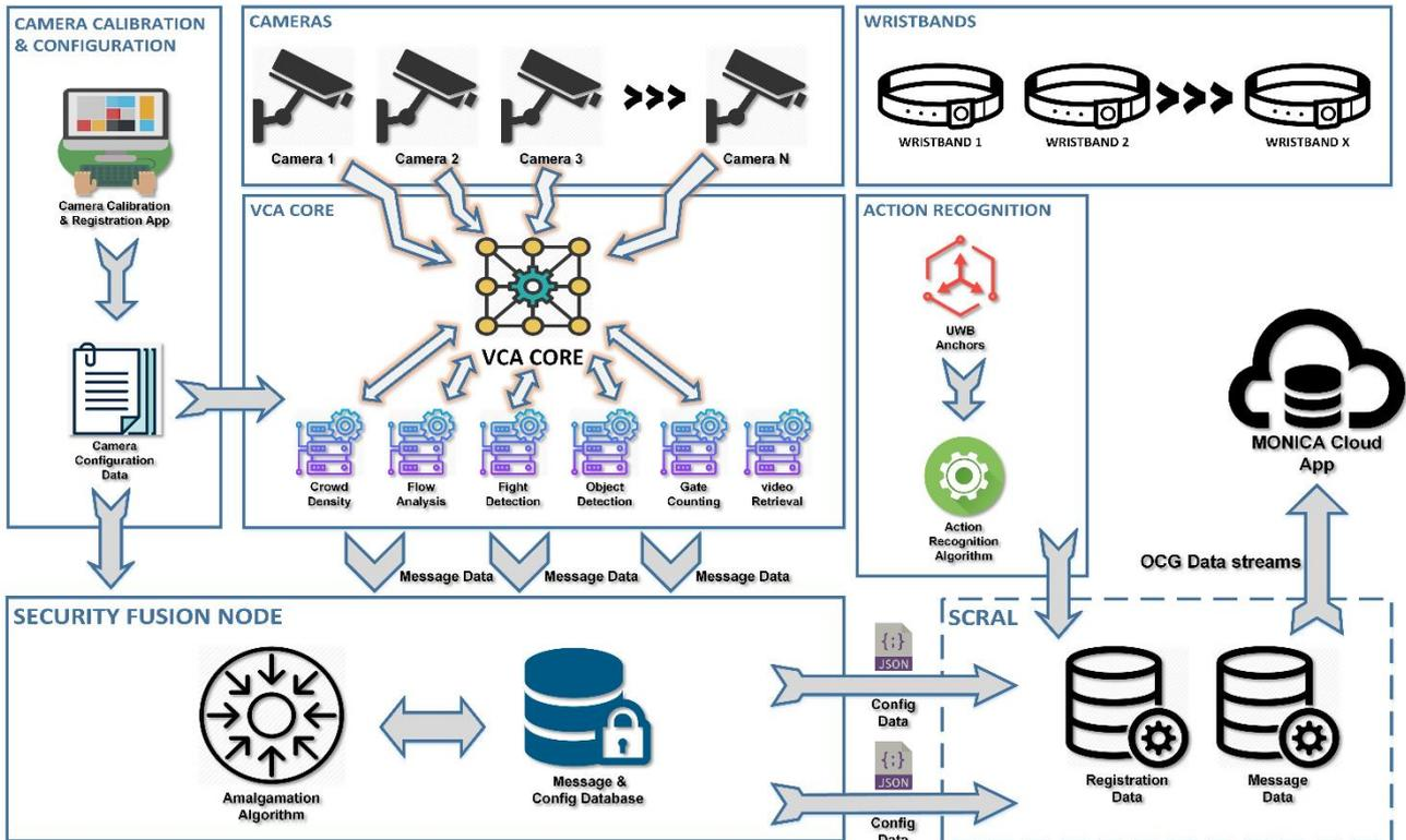
**Figure 2: Extrapolated view of the WP5 components with respect to the storage and use of models with the various detection algorithms. The proposed video retrieval algorithm sits in between VCA core and Security Fusion Node (SFN)**
