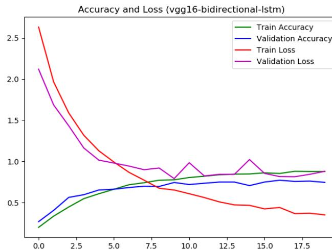
**Figure 14: Accuracy and Loss metrics of VGG16 + bidirectional LSTM over 20 epochs**
