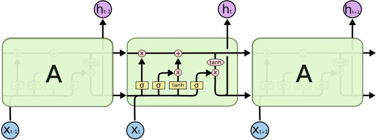
Figure 10: The repeating module in an LSTM contains four interacting layers
