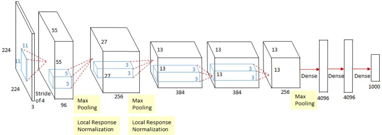
Figure 11: The CaffeNet CNN model is used to extract spatial features from each input frame.
